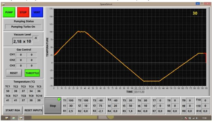
Screen shot of a run with NVSS-600, where table temperature profile, temperatures and vacuum level are displayed on the screen.
