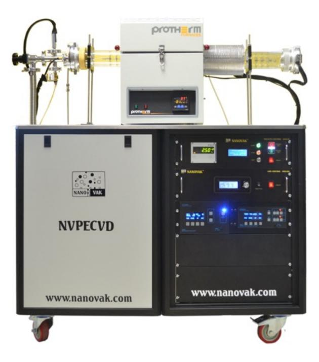
Nanovak Ar-Ge has recently developed PECVD (Plasma Enhanced Chemical Vapor Deposition) tube furnace system, which consists of 300W RF plasma source, optional split tube size furnace, 3 channel mass flow controller unit. It is ideal for TiN, TiC, SiC, Si<sub>3</sub>N<sub>4</sub>, Graphene film production.
